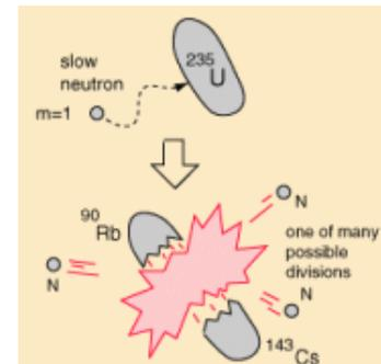
Neutrons produced in these reactions are fast neutrons – moving at 14,000 km/s or 31.3 million miles per hour.. A fast neutron will not be captured, so it must be slowed down by **moderation** to increase their capture probability in fission reactors. *A single fission event can yield over 200 million times the energy of the neutron which triggered it!*
